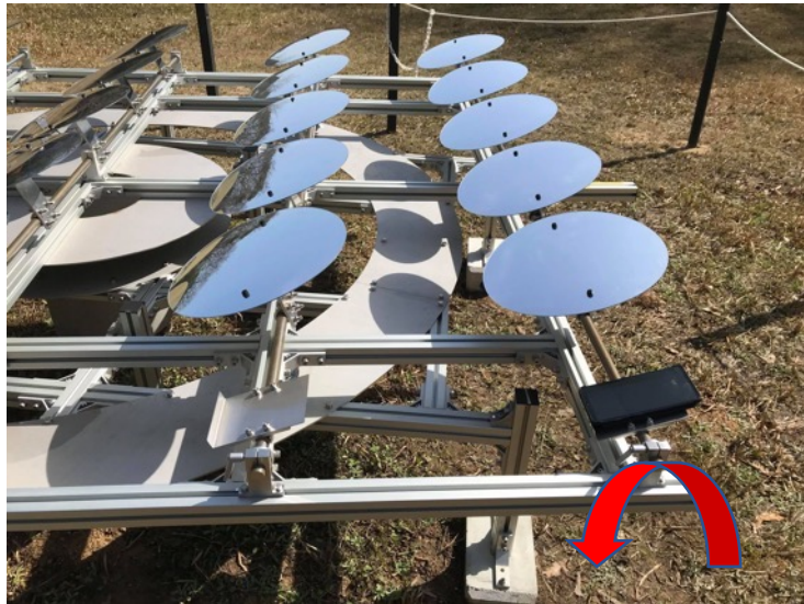
A key for tilt angle adjustment
